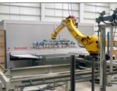
**At the Spanish collector manufacturer Hucu, a robot charges the Sunlaser welding unit.**
