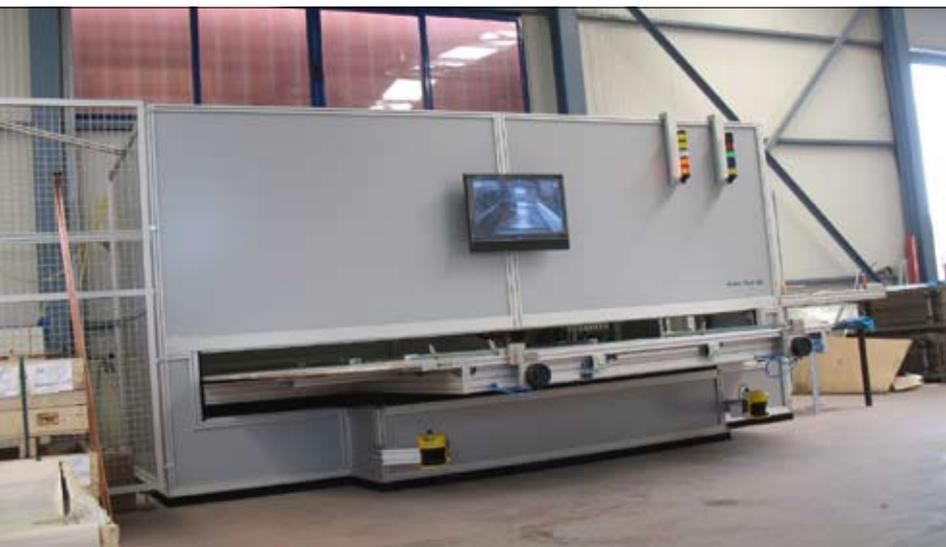
**Sunlaser produces welding systems in which a carousel transports the absorbers into the laser welding chamber.**
